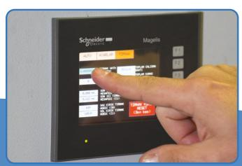
**HMI:** A touch panel is supplied with the take-up device to adjust all the settings.
