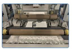
Automatic Roll Width Adjustment: The operator sets the fabric width from HMI and motorized fabric arms open or close to hold paper tube core.
