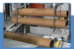
Pneumatic Heads for Fabric Centering: To hold paper core in place, fabric arms also have pneumatic heads which ensures that the paper tube core is always at the center and tightly held during rewinding operation.
