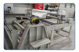
**Jumbo Roll Auto Loader/Unloader:** An auto loader is designed and developed for an efficient and non-stop operation. The rolls to be unwinded are placed into the auto loader and moved to the safety chuck position. Once the rolls are unwinded, the empty shaft is unloaded.
