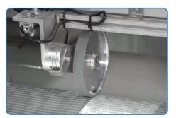
**Encoder Wheel:** For precise fabric length measurement, an encoder wheel is used. Feedback signals from the encoder drives the winder servo motors PID controller to make sure that even with extreme operating speeds, rewind stops at exactly right fabric length.
