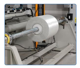
**Ultrasonic Sensor:** Accurate in mm range. Capable of measuring with a standing still roll. Infinite life. Invisible target point. No touching to the fabric.
