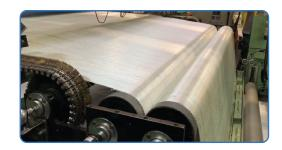
Measuring the traveling speed of the fabric during production is critical for the following winding or processing operations.
