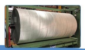
Programmable nip pressure is of high importance for tight roll winding. The applied pressure changes with roll lenght/weight. However, it a challenge to measure the nip pressure and use it to control the vertical pressure applied to the roll.
