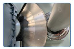
**PVC Shaft Guard:** For additional protection, steel shaft is covered with a PVC pipe which makes sure that the blade does not get in contact with the shaft.
