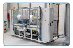
**Fully Automatic Operation:** Roll slitter is fully enclosed with glass barriers and operation is fully automatic.
