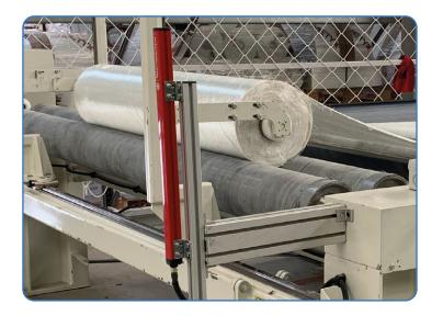
**Surface Unwinding:** The fabric roll is placed on to two surface roller driven with a motor. Since the weight of the roll is supported, the weight capacity of surface feeders are much higher compared to center feeders. Also, surface feeders ensure constant linear fabric speed with changing roll diameter without using an encoder or an ultrasonic sensor.
