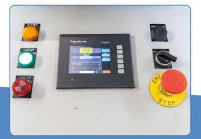
**HMI:** A touch panel is supplied with the feeder to adjust all the settings.
