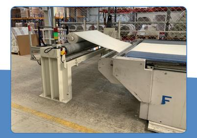
**Tension Control:** With fine adjustment of encoder pulses, the fabric tension can be kept constant without using a loadcell or pneumatic dancer.
