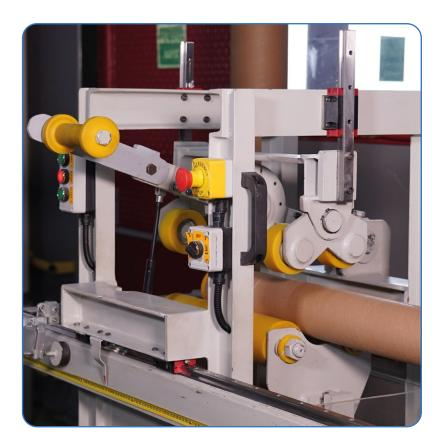
**Shaftless Design:** The cutter does not have a steel shaft. Thus, same machine can be used for either 3" or 6" diameter. Since the blade cannot get into contact with a steel shaft, blade lifetime is longer and maintenance costs are much lower.
