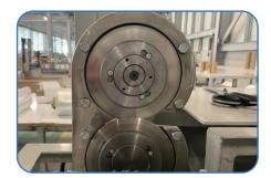
**Speed Control:** The single motor design controls not only the linear traveling speed but also the rotational blade speed.
