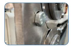
**Overlapping Control:** Blades overlapping distance can be set mechanically.
